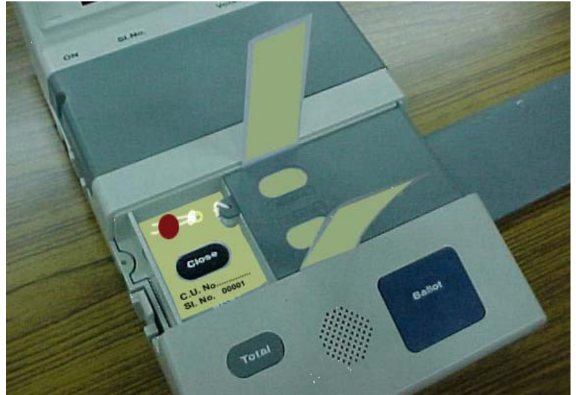
Sealing the inner door with Special Tag ECIL Machine
